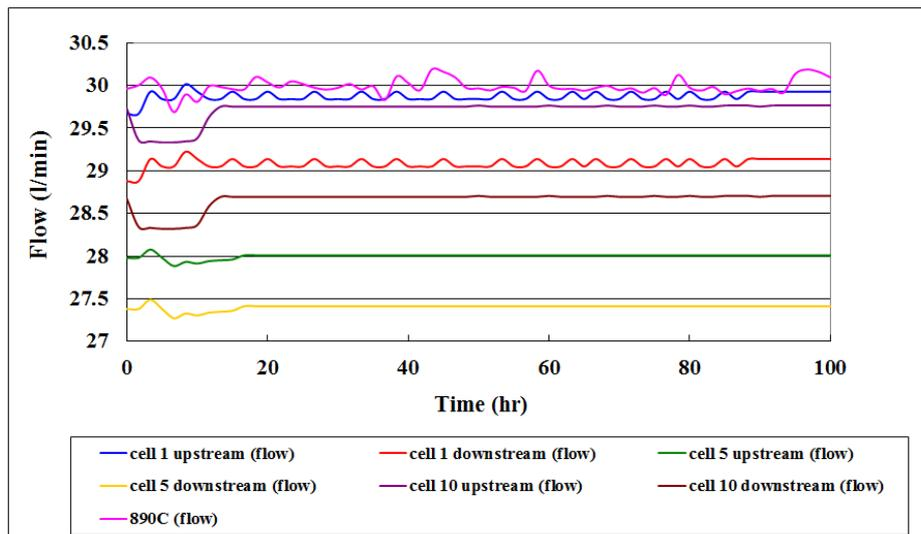
Fig. 5 Comparison diagram of local flow in different cells
