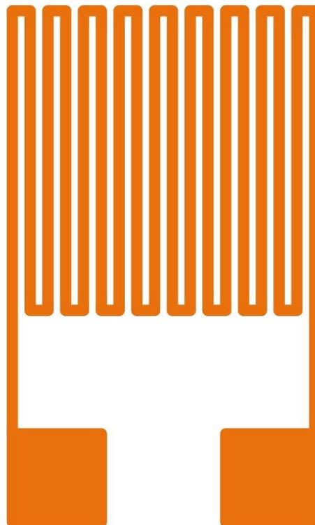
Fig. 1 Schematic diagram of design of micro temperature sensor
