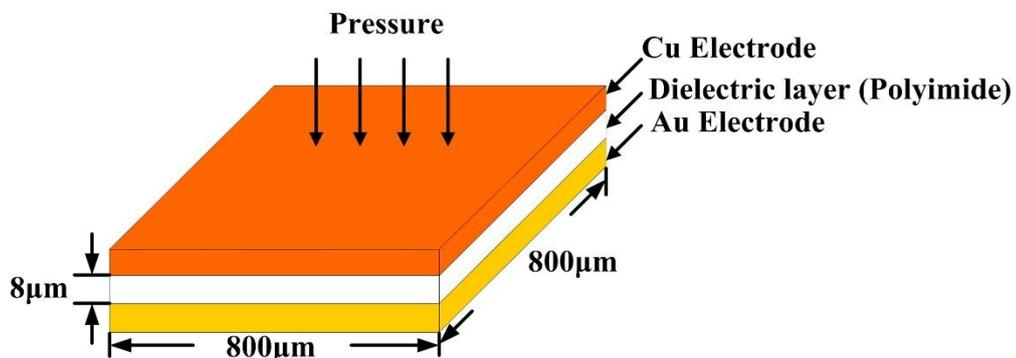
Fig. 3 Schematic diagram of design of capacitive micro pressure sensor
