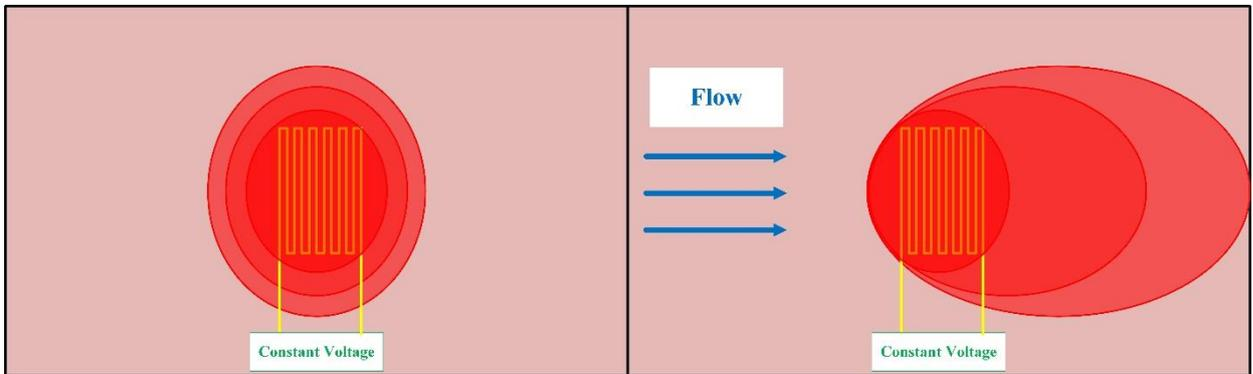
Fig. 2 Schematic diagram of sensing principle of micro flow sensor
