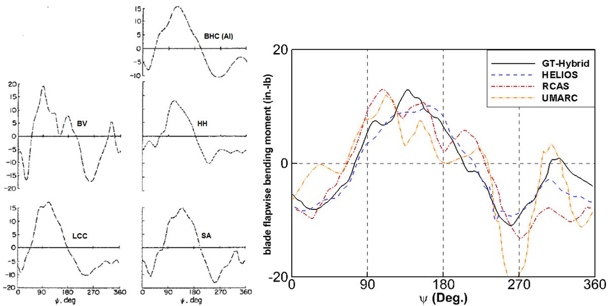
Fig. 7 Comparison of blade flapwise bending moment ( $\times 10^{-3}$  in.-lb) vs azimuth;  $r=0.5R$
