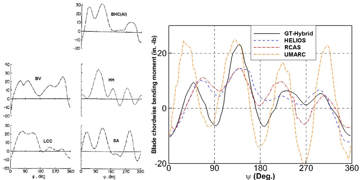
Fig. 8 Comparison of blade chordwise bending moment ( $\times 10^{-3}$  in.-lb) vs azimuth;  $r=0.5R$  (Left : 1974, Right : Present)
