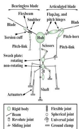
Fig. 2 Schematic of helicopter rotor model in DYMORE
