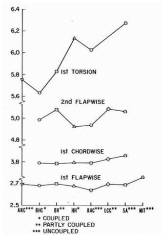
Fig. 3 Comparison of 1974 rotor blade rotating natural frequencies in vacuo (per rev.) at 100% nominal rotor speed, collective pitch = 0 deg
