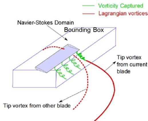
Fig. 1 Schematic of hybrid methodology
