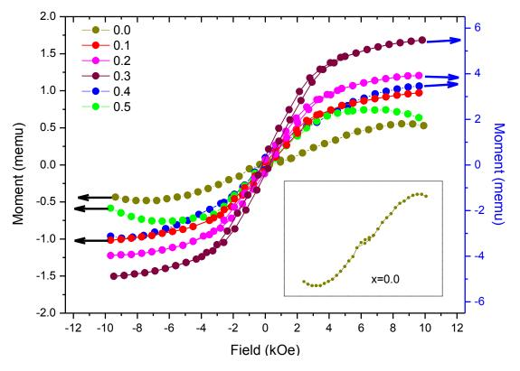
Fig. 3 M-H curves for undoped and doped BiFeO<sub>3</sub>
