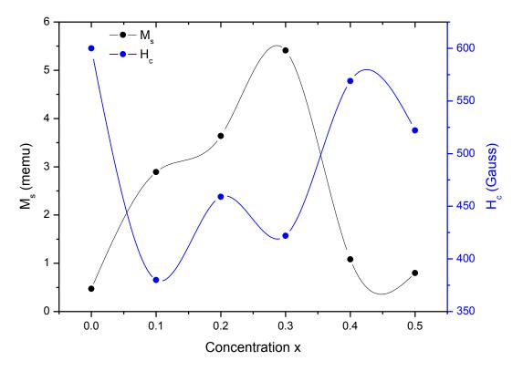
Fig. 4 Saturation magnetization and coercivity as a function of dopant concentration
