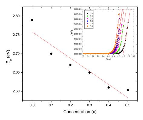
Fig. 2 Band gap of Bi<sub>1-x</sub>La<sub>x</sub>FeO<sub>3</sub> films as a function of lanthanum concentration
