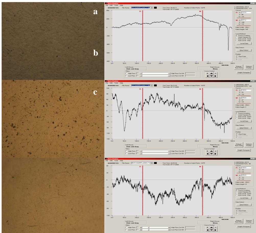
Fig. 3: Optical images (at 50x) and surface profile of (a) SS420 (b) SS 304, and (c) SS 201 showing smooth surface after polishing
