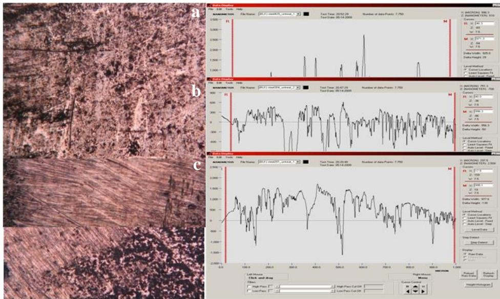
Fig. 2: Optical images (at 50x) and surface profile of (a) SS420 (b) SS 304, and (c) SS 201 showing surface roughness before polishing
