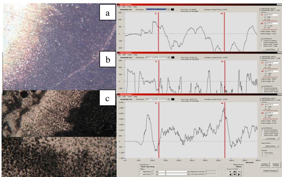
Fig. 4: Optical images (at 50x) and surface profile of (a) SS420 (b) SS 304, and (c) SS 201 showing surface roughness/nucleation sites after etching
