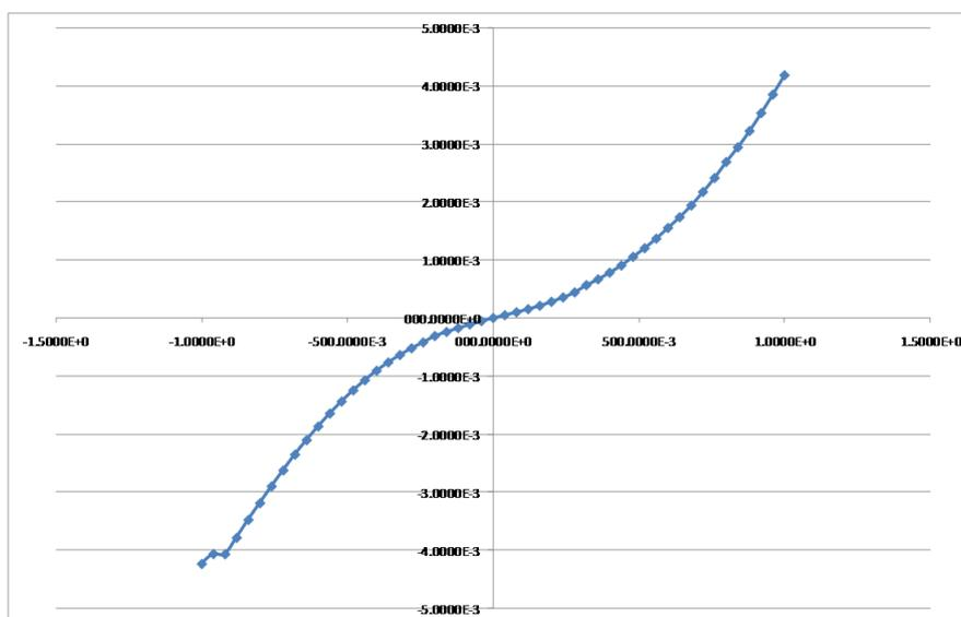
Fig. 7 I-V characteristics of iron oxide coated carbon nanotubes
