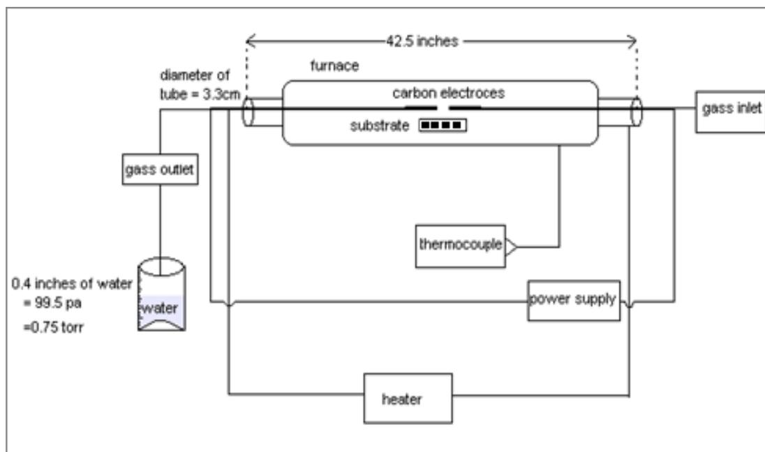
Fig. 1 Block diagram of home-made setup of Plasma Enhanced CVD
