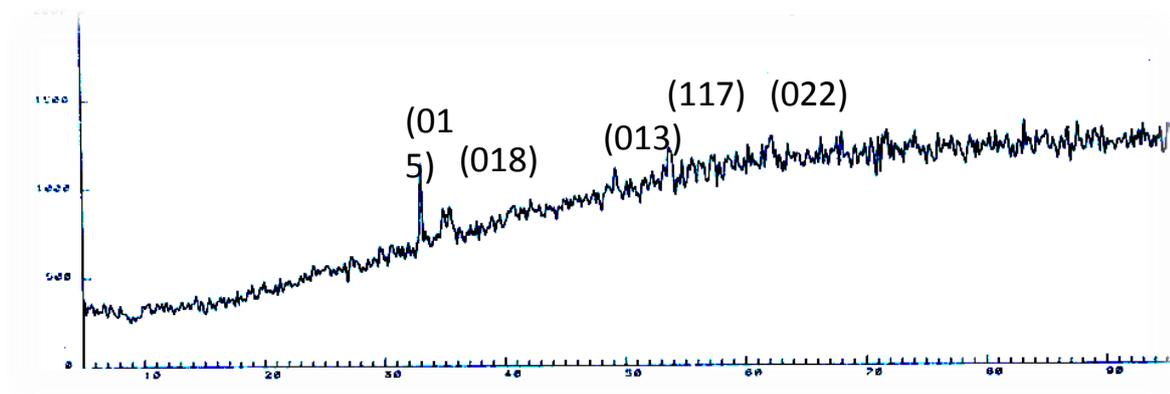
Fig. 6 XRD result of iron oxide coated carbon nanotube
