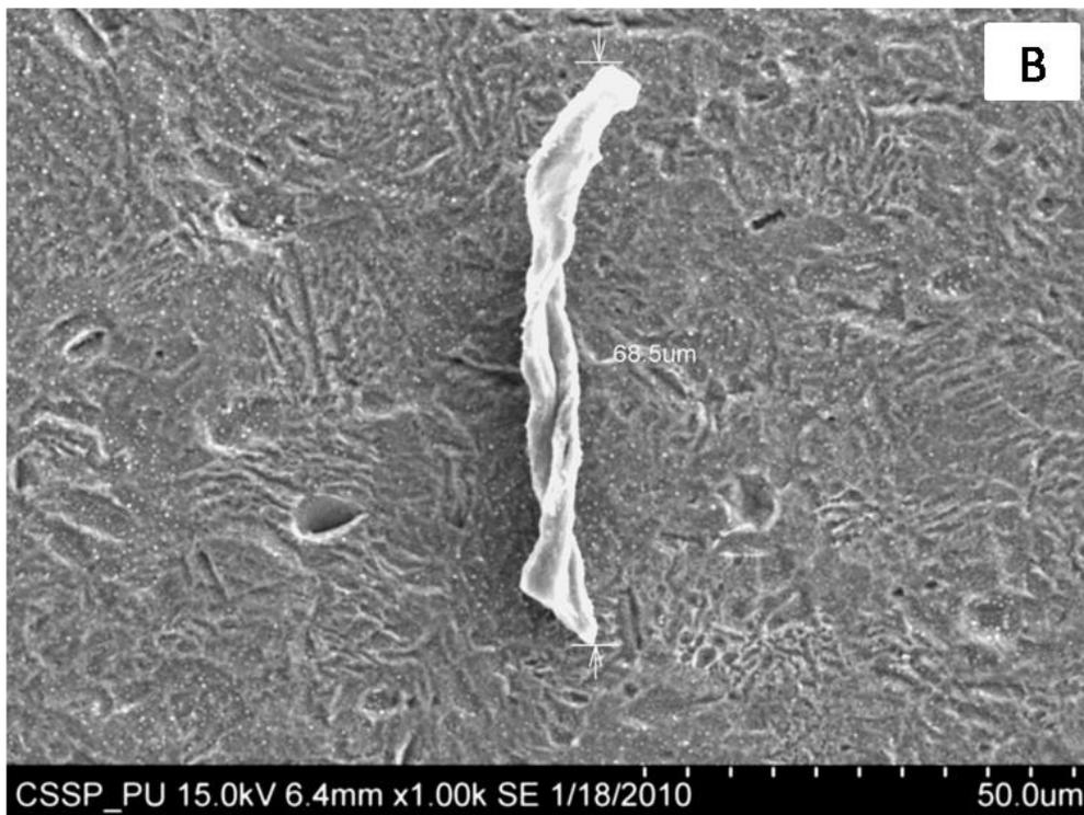
Fig. 5 SEM image iron oxide NPs coated bundles of Carbon nanotube
