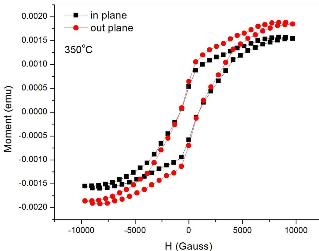
Fig. 2 Room temperature M-H curve for AlFeO<sub>x</sub> thin film annealed at 350°C.
