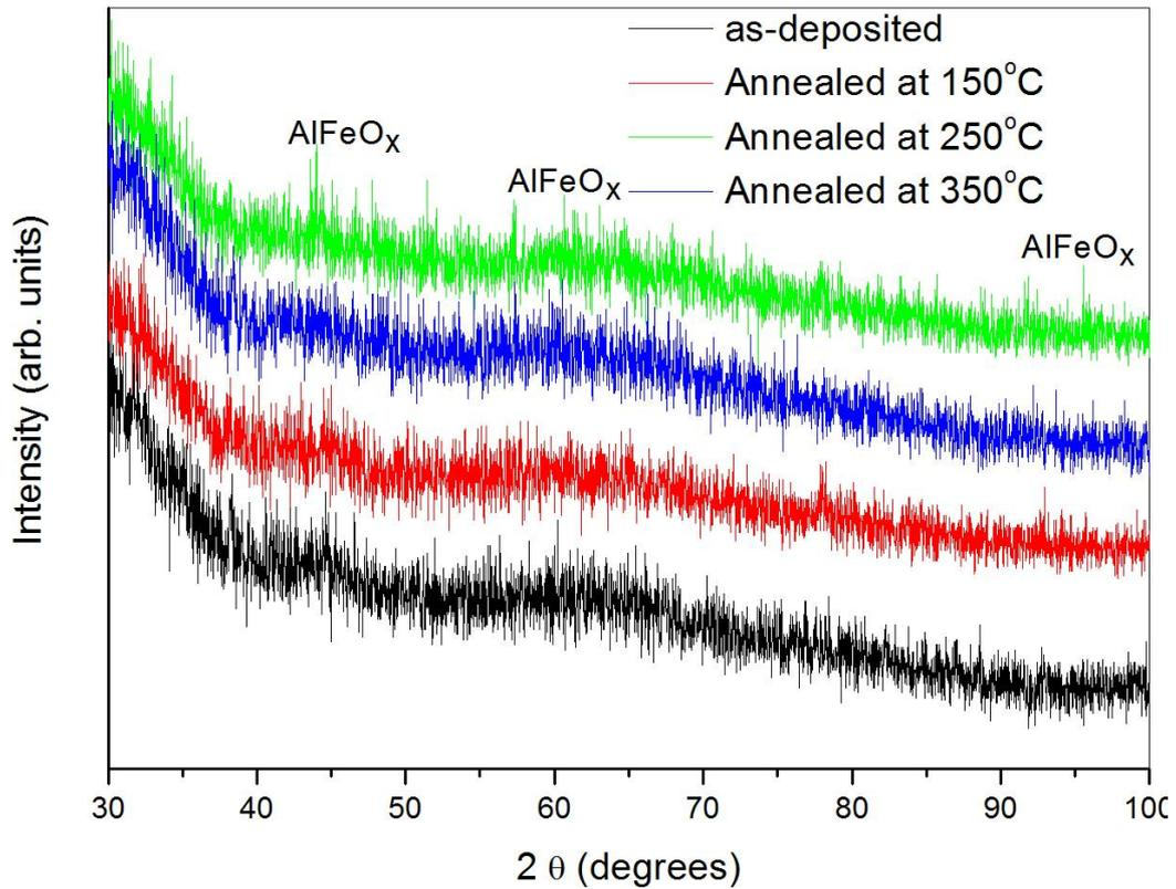
Fig. 1 XRD pattern of AlFe<sub>2</sub>O<sub>x</sub> thin films oxidized at oxygen flow rate of 10sccm and annealed at 150°C, 250°C and 350°C.
