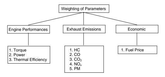
Fig. 2 AHP model for deriving the weightages of parameters
