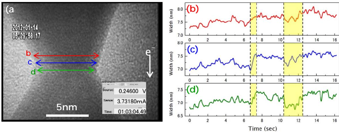
Fig. 3 (a) TEM image of a gold nanowire, and (b)-(d) time variation of the wire width.
