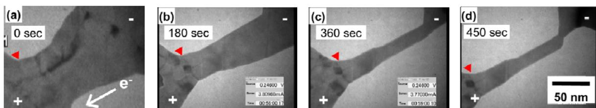
Fig. 1 TEM movie during narrowing process of an Au nanowire. Electrons flow from the right-top to the left-bottom as indicated by an arrow in (a). Plus and minus signs denote the voltage polarity. Positions indicated by red arrows correspond to each other.
