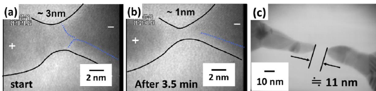
Fig. 4 (a)-(b): Images during the rupture process, and (c): fabricated nanogap.
