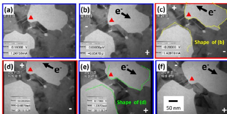
Fig. 2 Geometrical change during alternation of the current flow. Positions indicated by
