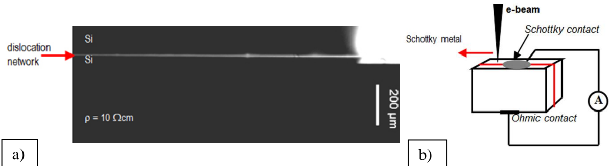
Fig. 3 Formation of a conducting channel along the dislocation network in the interface of a bonded Si wafer pair (a). EBIC micrograph. Sketch of the experimental setup (b).
