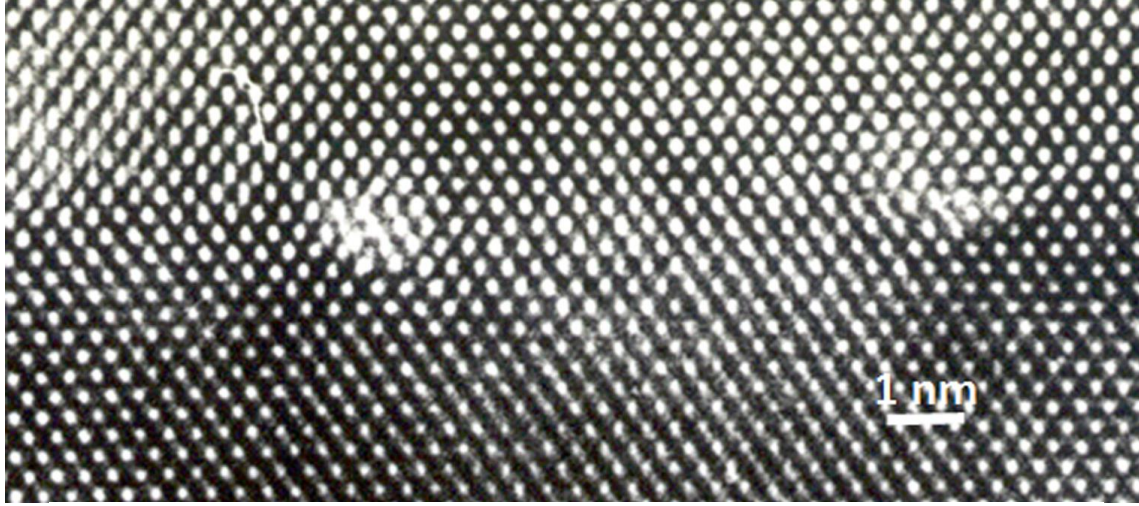
Fig. 1 Cross-section image ( \{110\} plane) of two screw dislocations in silicon. The diameter of the dislocation cores is about 1 nm. High-resolution electron microscope (HREM) image.
