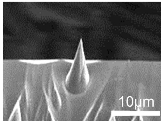
Fig. 2 SEM image of a needle formed upon a Si substrate by ion-shadow method
