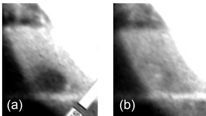
Fig. 8 TEM image after resistive switching of (a) HRS to LRS and (b) LRS to HRS.
