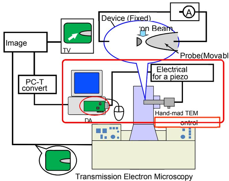
Fig. 3 Schematic image of the in-situ TEM experimental system
