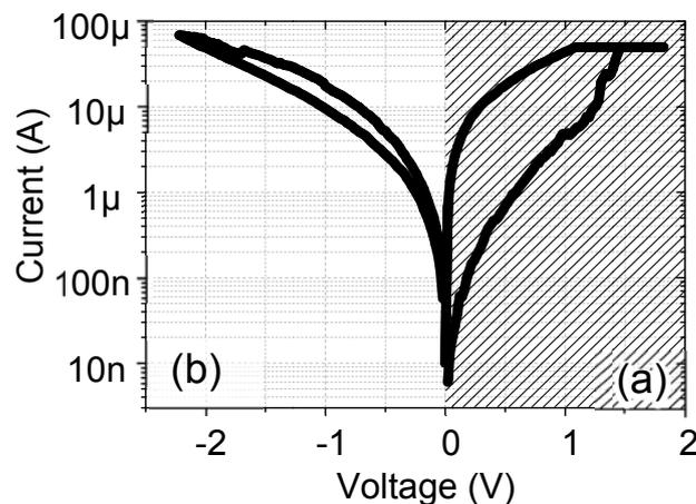
Fig. 7 I-V characteristics obtained during ReRAM operation.
