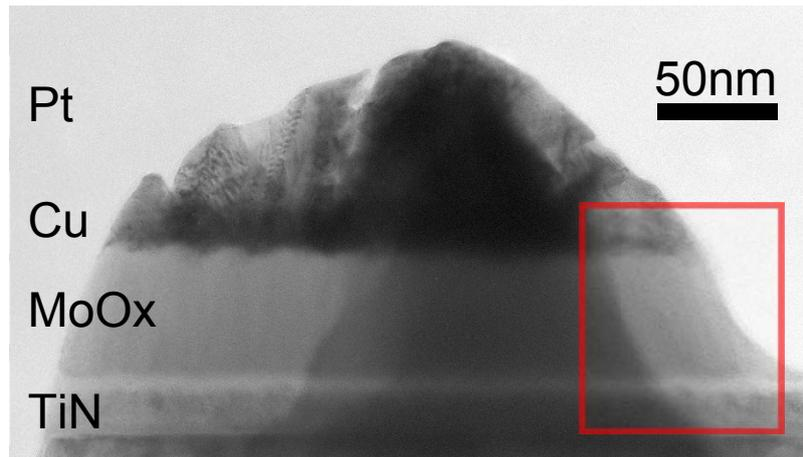
Fig. 6 TEM image of a Pt/Cu/MoOx/TiN miniaturized ReRAM device in initial state. Red boxed area shows the magnified position in Figure 8.
