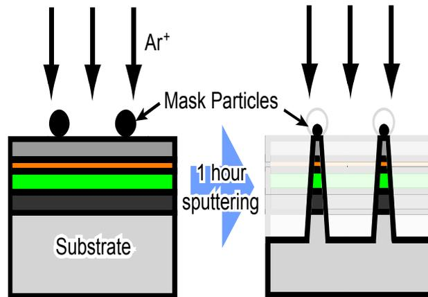
Fig. 1 Schematic image of the ion-shadow method
