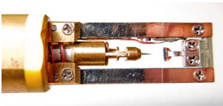
Fig. 4 TEM specimen holder with a piezo actuator
