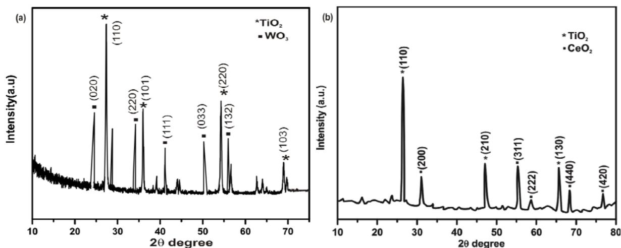
Fig. 1 XRD pattern of (a)  $WO_3$ - $TiO_2$  and (b)  $CeO_2$ - $TiO_2$  nanoparticles
