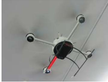
Fig. 1 The md4-200 quadrotor helicopter of microdrones equipped with Galaxy S3 during flight
