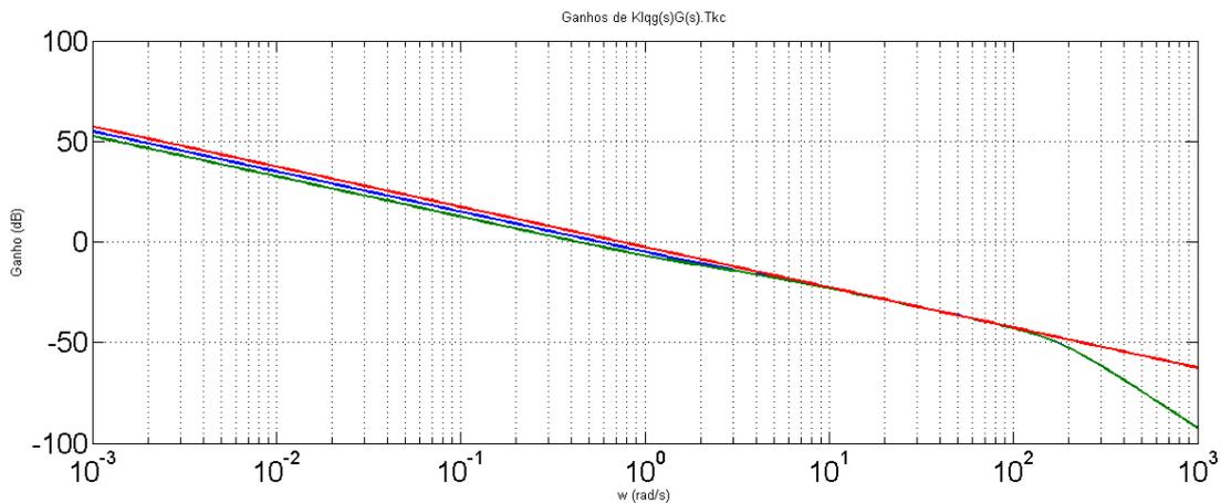
Fig. 4 Frequency gains of the open loop system with controller added
