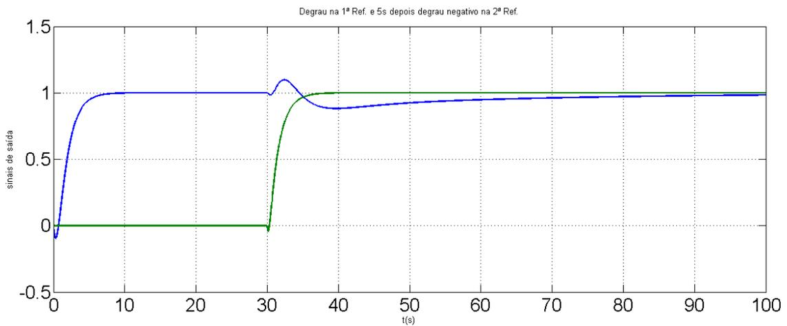
Fig. 6 Step responses of the controlled system, with the blue line representing the first input and green line the second
