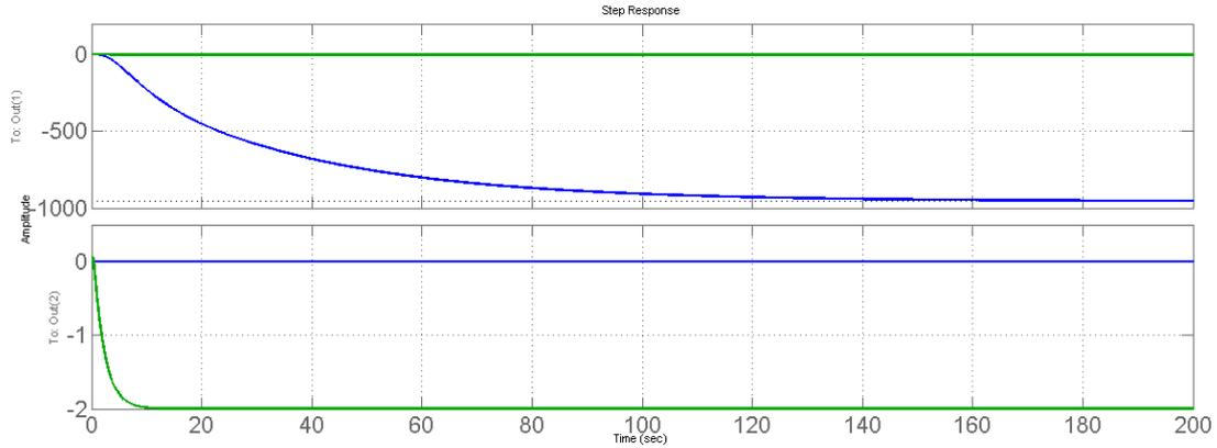
Fig. 2 Step response of the system, being applied in  $U_1$  (upper graphic) and  $U_2$ . The blue line represents output 1 (Paralysis) and green line output 2 (MAP)
