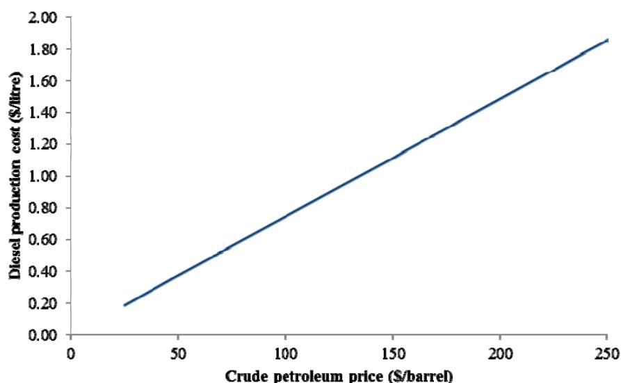
Fig. 3 Diesel fuel production cost as a function of crude petroleum price
