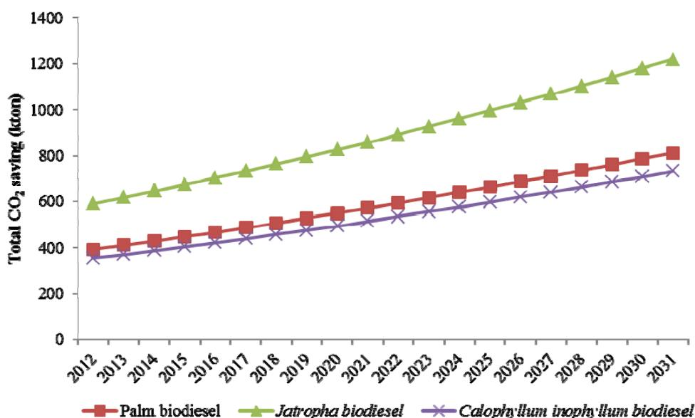
Fig. 2 Impact of CO<sub>2</sub> saving from 5% biodiesel substitution for diesel consumption
