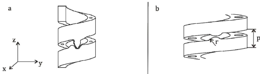
Fig. 2 schematic view of contours for the helix. Involute (a) and unrolling circles (b)
