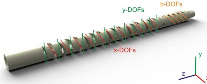
Fig. 4 Layout for the S-like bending with planar base joints
