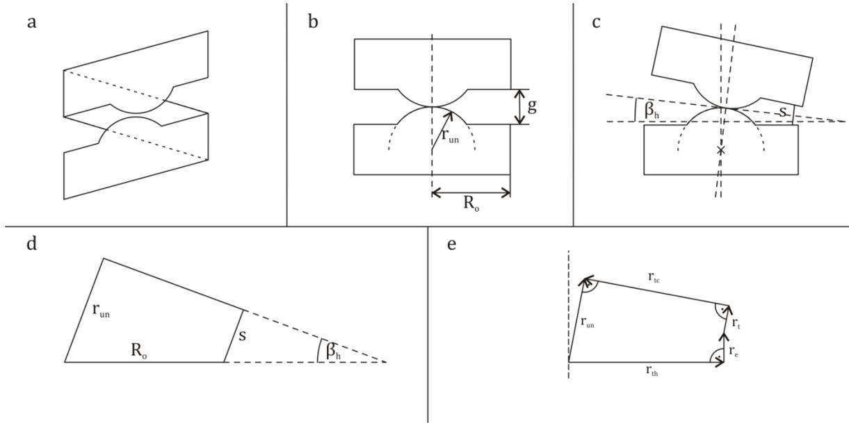
Fig. 5 Schematic view of helical joint (a), simplified model (b), half bending angle  $\beta_h$  and tendon lengths (c), approximation (d) and closed vector chain (e)
