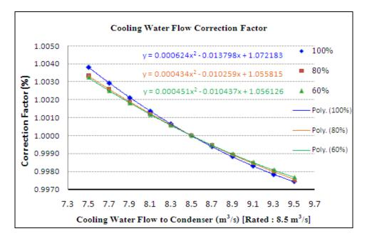
Fig. 4 Correction factor at various cooling water flow to condenser.
