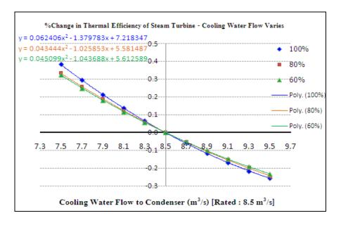
Fig. 3 The %change in thermal efficiency of steam turbine at various cooling water flow to condenser.
