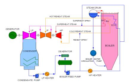
Fig. 2 Power plant cycle for 300 MW.
