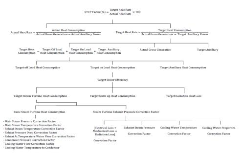
Fig. 1 Calculation diagram for STEP factor.
