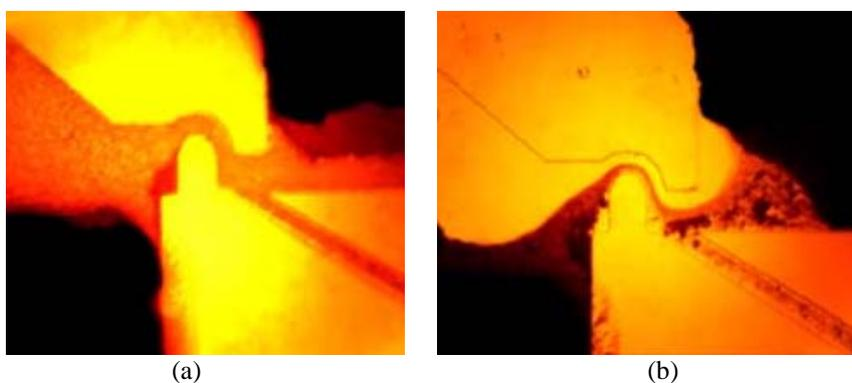
Fig. 3 Sample flow patterns on the Lab-on-a-Chip; (a) standard hematocrit and (b) lower standard hematocrit.
