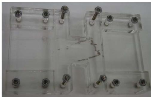
Fig. 2 A new-acrylic-plate set; H shape, used in the current work.
