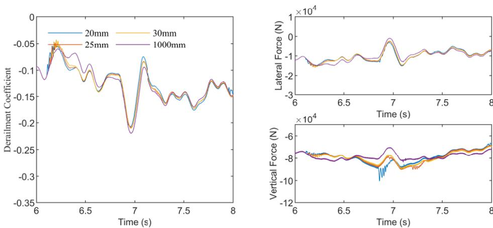
Fig. 4 The wheel response when PGA is 0.3g
