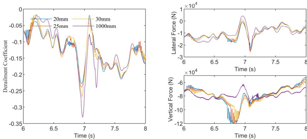
Fig. 5 The wheel response when PGA is 0.5g
