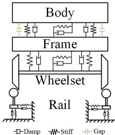
Fig. 1 Train-rail coupling system model
