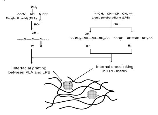
**Scheme 1.** Mechanism of the reactive blending of LPB in PLA matrix.
