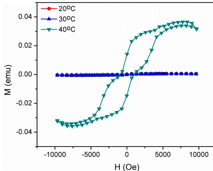
Fig. 3 M-H curves for iron oxide nanoparticles
