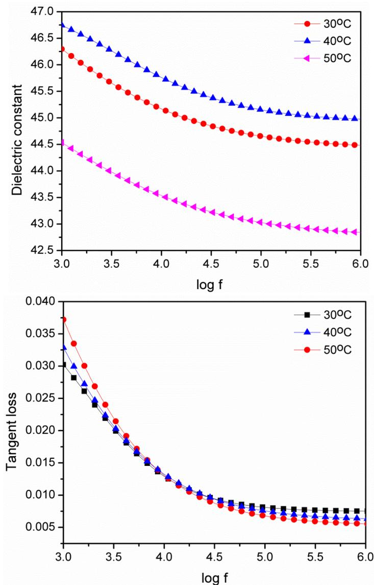
Fig. 2 Dielectric constant and tangent loss for iron oxide nanoparticles
