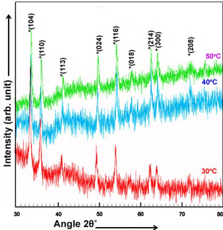
Fig. 1 XRD patterns for iron oxide nanoparticles prepared with variation in solution temperature
