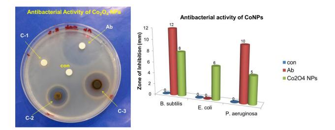
Fig. 3 (left) *B. subtilis* zones of inhibition (ZOI) around cobalt oxide nanoparticles impregnated disks. The distance of the bacterial lawn from disk can clearly be noticed, (right), graphs showing the results of ZOI formed around the highest particles concentration (C-3) soaked disks against B. subtilis, E. coli and P. aeruginosa.
