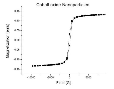
Fig. 2 Magnetization versus magnetic field plot of as prepared cobalt oxide nanoparticles at room temperature displaying the ferromagnetic nature of particles.
