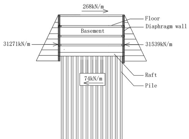
Fig.5 Horizontal loadings distribution
