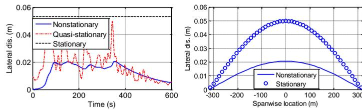
Fig 4. RMS displacements: (a) at middle center; (b) along bridge deck
