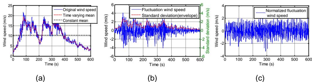
Fig 2. Full-scale wind speed: (a) longitudinal wind speed and mean; (b) longitudinal fluctuation wind and standard deviation; (c) longitudinal normalized fluctuation wind
