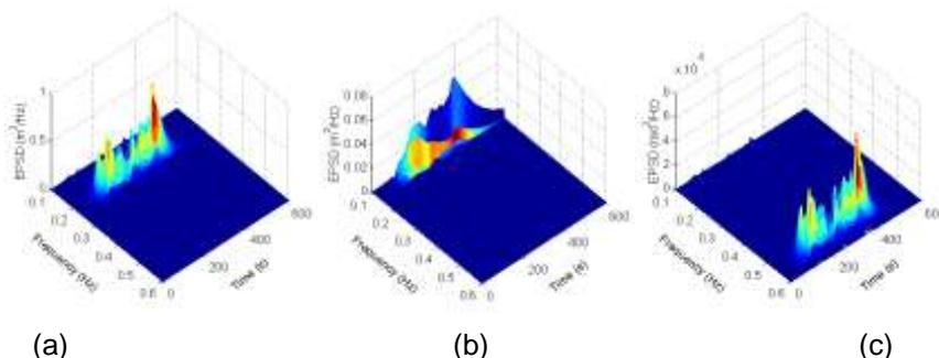
Fig 3. EPSD of main girder displacements at middle center: (a) vertical displacement; (b) lateral displacement; (c) torsional displacement
