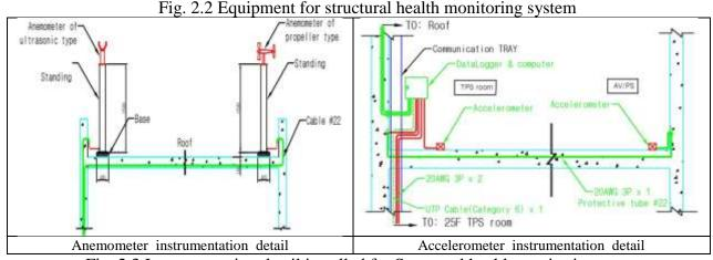
Fig. 2.3 Instrumentation detail installed for Structural health monitoring system
