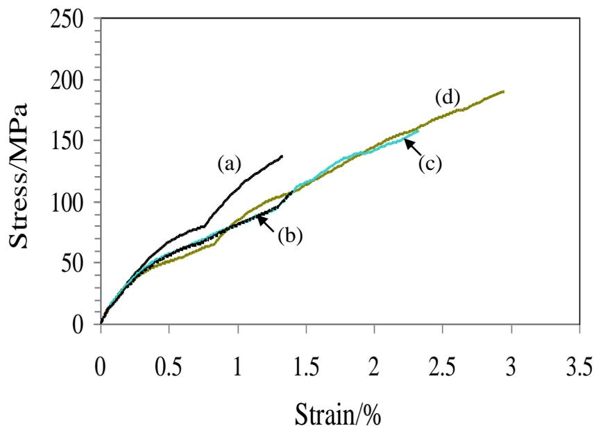
Fig.4 Stress-strain curves from tensile testing of (a) only Mg alloy, (b) untreated carbon fiber reinforced magnesium alloy composites, (c) Cu-Ni-C magnesium alloy composites, (d) composites of (c) fluorinated at 100°C.
