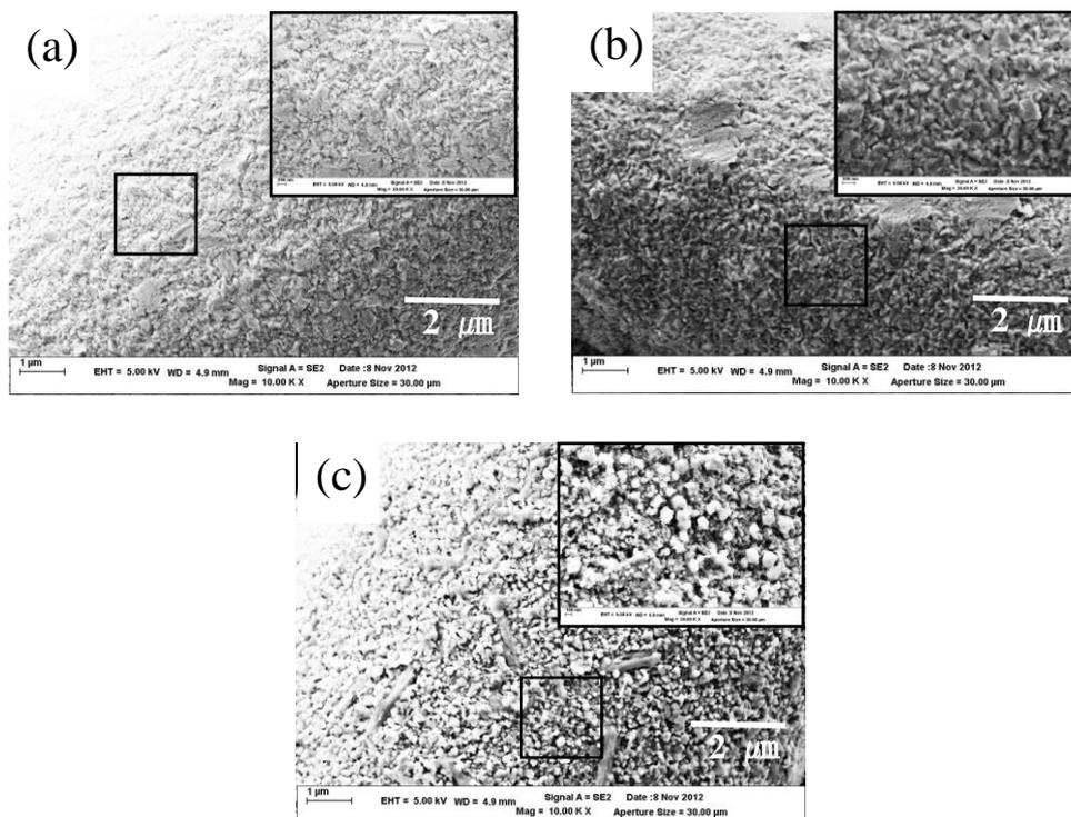
Fig.2 SEM images of Cu-Ni-C fibers prepared with (a) untreated, (b) fluorinated at 25°C, and (c) fluorinated at 100°C.
