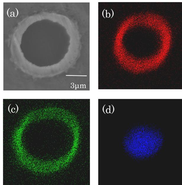
Fig.1 SEM image (a) and mapping images ((b)Ni, (c)Cu and (d)C) of Cu–Ni duplex layers coated on carbon fiber in cross-section of magnesium composite matrix.
