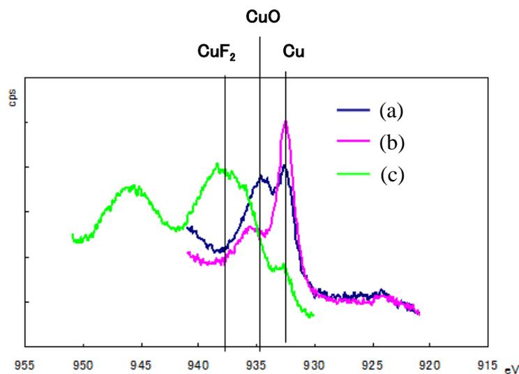
Fig.3 XPS spectra of Cu 2p for various samples prepared with (a) untreated, (b) fluorinated at 25°C, and (c) fluorinated at 100°C.
