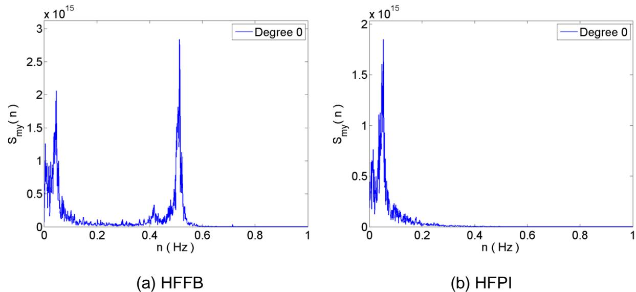
Fig.9 PSD of base moment at 0° wind attack angle
