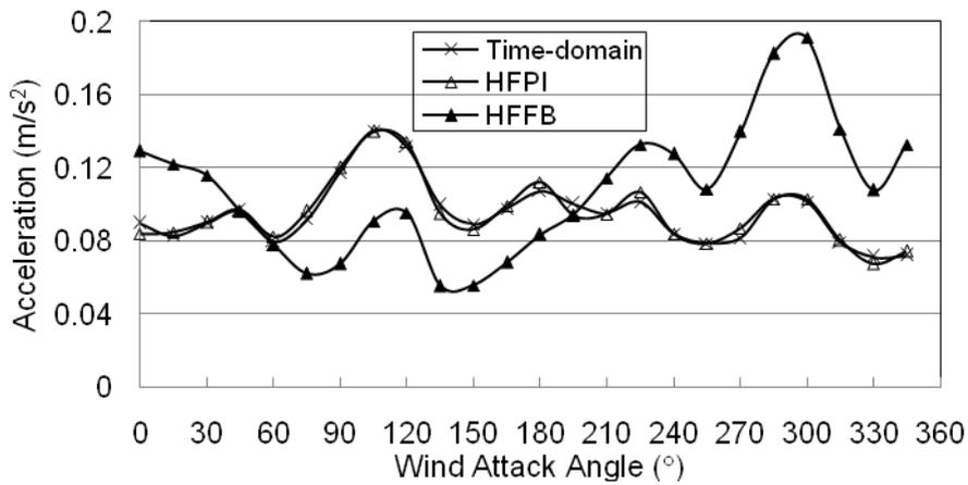
Fig. 4 Torsional acceleration responses
