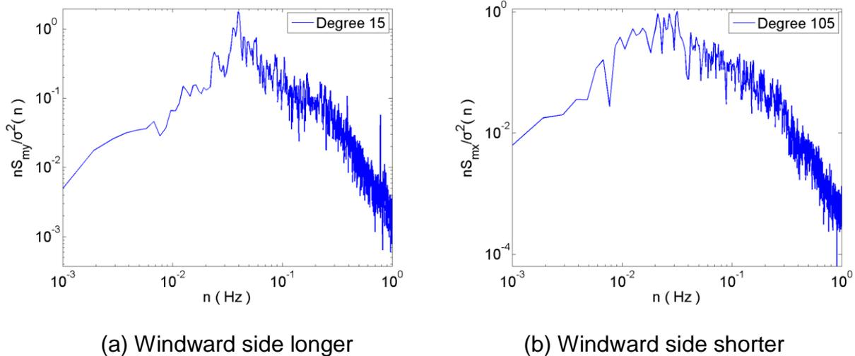
Fig. 11 Normalized PSD of across-wind base bending moment
