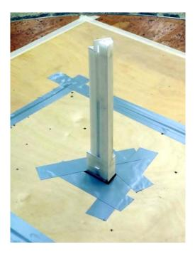
Fig. 1 HFBB tests for a 30-story building
