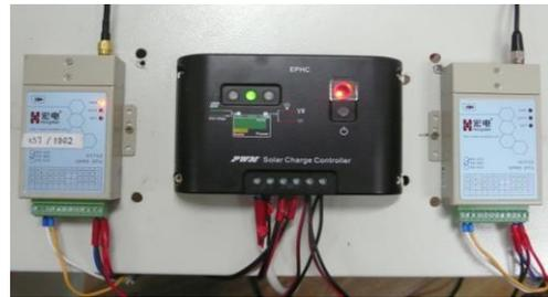
Fig. 3 RTU modules used in the field
