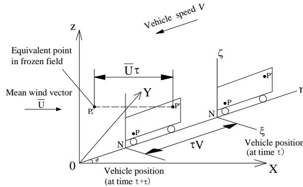
Fig. 1 Two points moving with the vehicle and equivalent point (Cooper, 1984)
