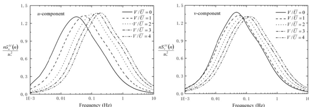
Fig.3 The influence of speed ratio on power spectra of  $u$ - and  $v$ -components
