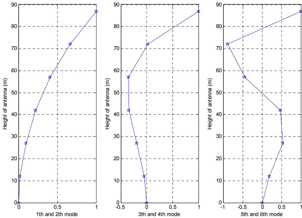
Fig. 3 Vibration modes of the antenna
