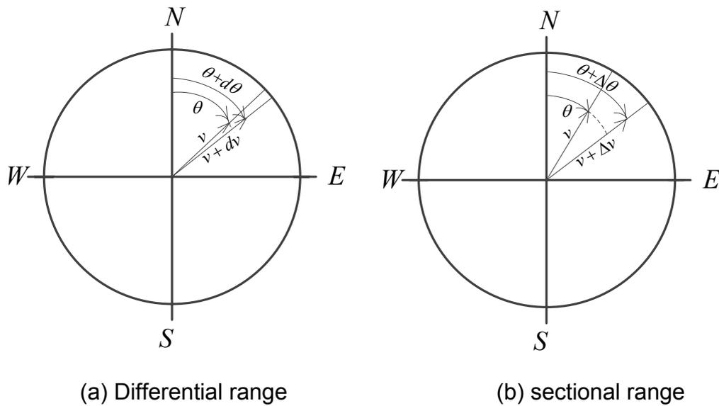
Fig. 1 Differential range of wind speed and direction plane
