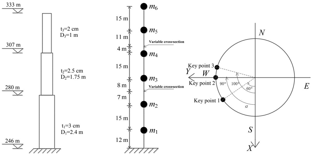
Fig. 2 A steel antenna
