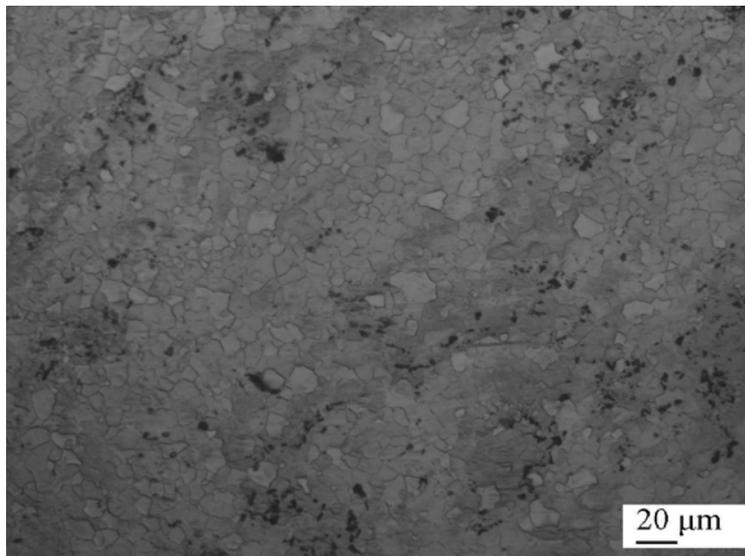
Fig. 5: Microstructure of the specimen deformed at 350 °C/10 s<sup>-1</sup> (Domain #3).
