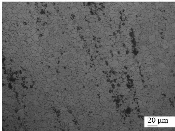
Fig. 3: Microstructure obtained on the specimen deformed at 300 °C/ 0.0003 s<sup>-1</sup>.
