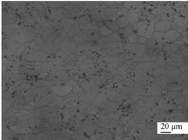
Fig. 4: Microstructure obtained on the specimen deformed at 450 °C/ 0.0003 s<sup>-1</sup>.
