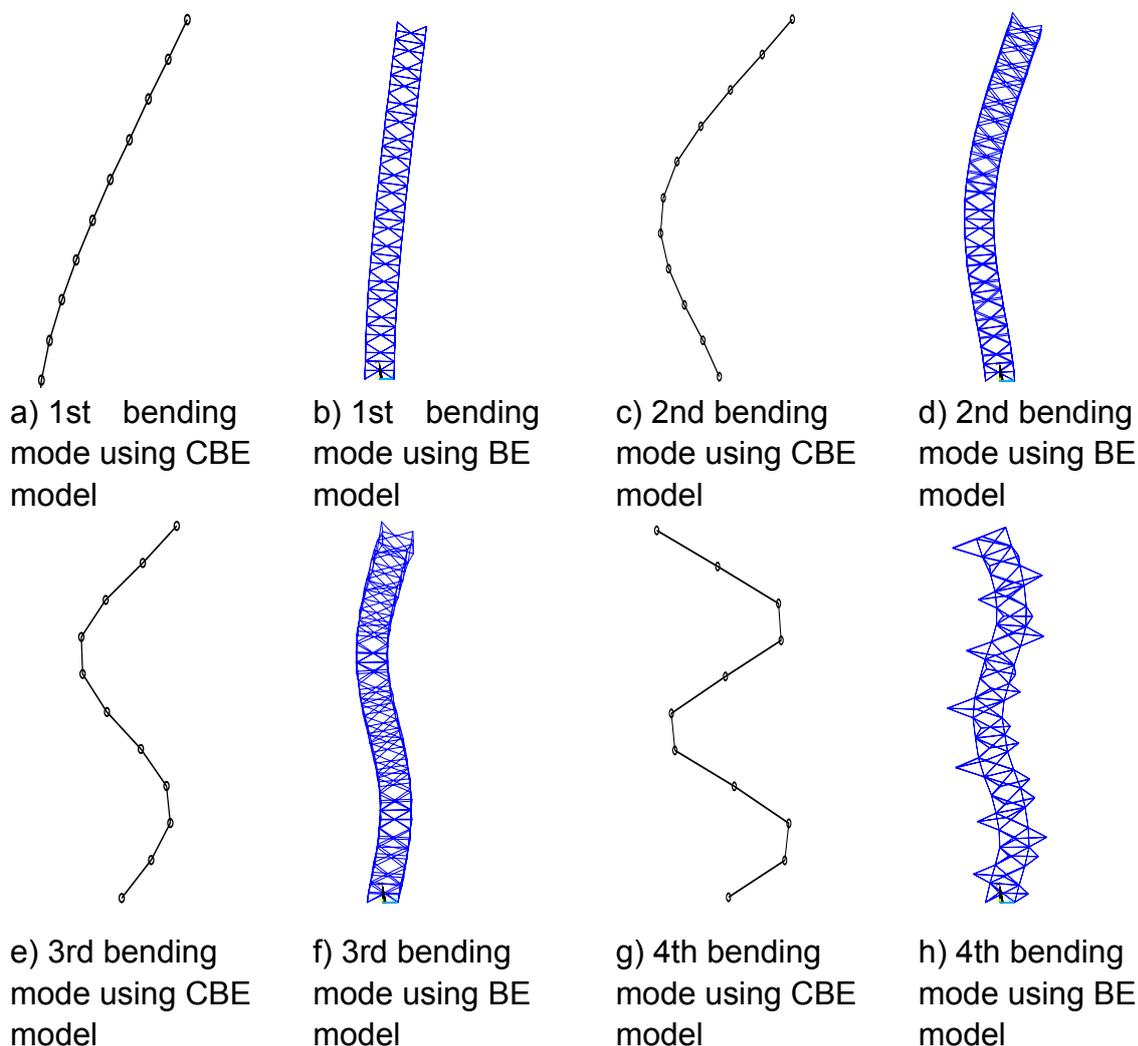
Fig. 3 Mode shape comparison between the continuum-beam-element (CBE) model and the bar-element (BE) model of the tower crane
