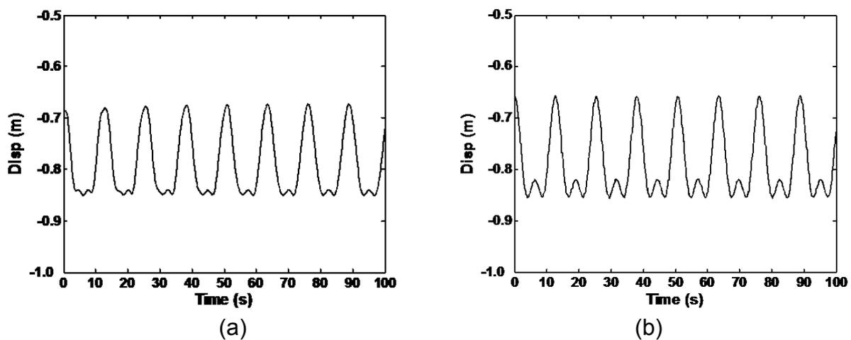
Fig. 6 Tip displacement responses of the tower crane due to planar pendulum motion of the payload (a) without and (b) with considering the crane-payload interaction
