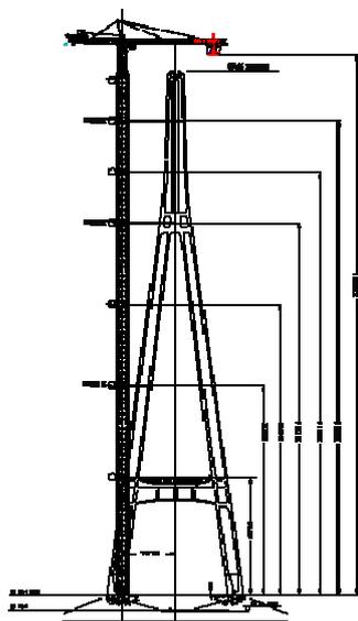
Fig. 1 Cable pylon - tower crane system of Sutong Bridge
