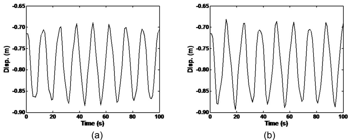
Fig. 5 Tip displacement responses of the tower crane due to spherical pendulum motion of the payload (a) without and (b) with considering the crane-payload interaction
