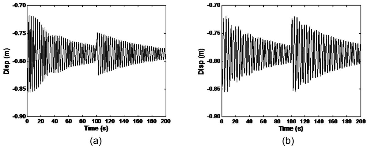
Fig. 4 Tip displacement responses of the tower crane during payload lifting (a) without and (b) with considering the crane-payload interaction
